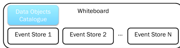
Figure 2. The Whiteboard can be thought as a group of Event Stores. The calls to the Whiteboard are dispatched transparently to the single Event Stores using the information in the Execution Context.
